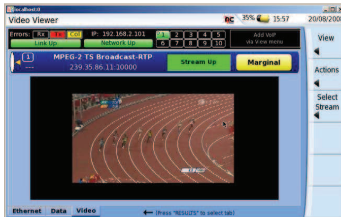
Figure 4: Example of IPTV Video Stream test
