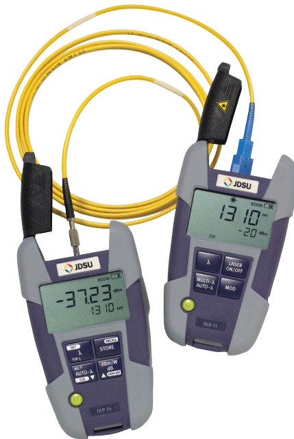
SmartPocket OMK-3x optical test kits include an OLS-3x optical light source, an OLP-3x optical power meter, and accessories
