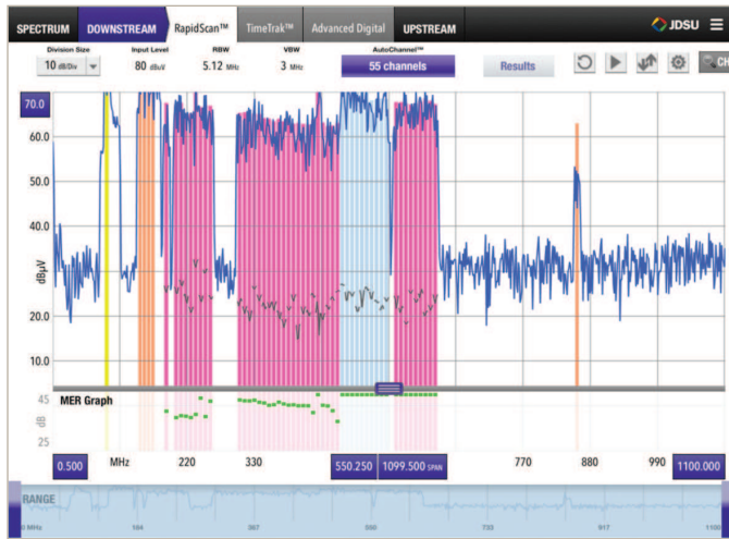
Full downstream channel scan screen
