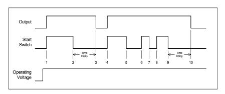
load. The *Initiate Switch* opens and closes at times #5, 6, 7, and 8, but re-closes before the end of the timing period keeping the *Output* ON and the load energized. At time #9 the Initiate Switch opens and remains open longer than the timing period causing the Output to turn OFF at time #10.
