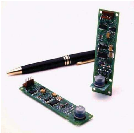
Models 901 (horizontal) and 902 (vertical) Biaxial Clinometers.
