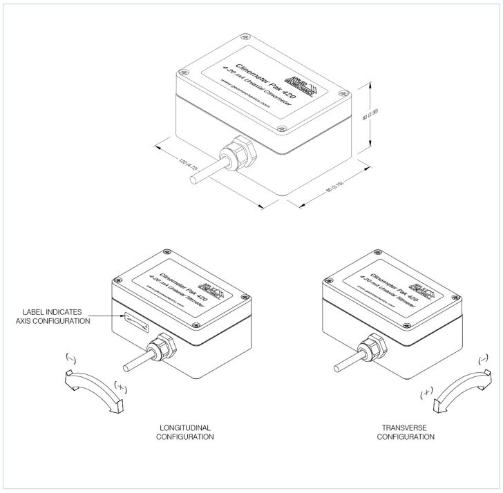
Clinometer is available with either longitudinal or transverse tilt configuration.
