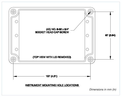
Mounting holes are accessed by removing lid of clinometer. Use 8-32 or 4 mm screws.
