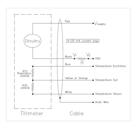
The Clinometer Pak 420 current signal is measured indirectly using a shunt resistor, R. Ohm's Law states that V1
