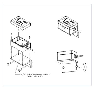
For mounting on vertical surfaces: Order the 81439 Mounting Bracket Assembly, which includes complete hardware.
