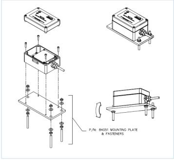
For mounting on horizontal surfaces: Screw the clinometer directly to the surface, or order the 84051 Mounting Plate Assembly, which includes complete hardware.
