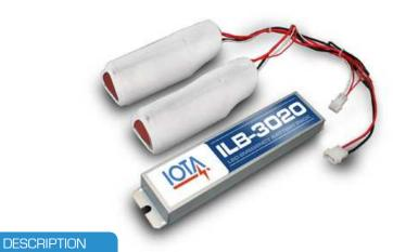
The **ILB-3020 750mA** from IOTA Engineering is a UL Recognized LED emergency battery pack that allows the same LED fixture to be used for both normal and emergency operation. In the event of a power failure, the **ILB-3020 750mA** switches to the emergency mode and operates the existing fixture for **90 minutes**. The unit includes one 16-cell or
