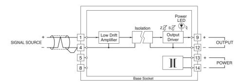
The M2VF3, by its fast-response feature, is not designed to eliminate noise present in the input signal. Use a shielded twisted-pair cable to prevent noise from entering through the input wiring.
