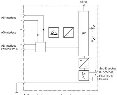
At the cable for power supply no slaves or repeaters may be attached.
