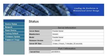
**Network:** You can change the network settings according to your network specifications. If you would like to give the Parallel Server a static IP address, you will need to Disable DHCP in the DHCP Setting menu. Once DHCP is disabled, enter the desired IP address on the "**IP Address**" field along with the "**Subnet Mask**" and click the "**Submit**"
