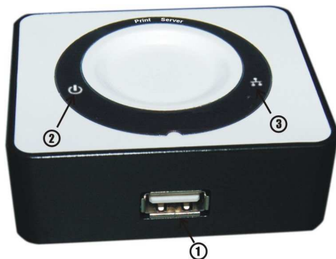
① USB Port ② Power LED ③ Ethernet LED
