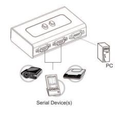
Figure 2: Serial Device + Serial Device to PC
