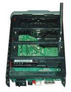
Align the edges of the hard drive platform and carefully slide the assembled platform into the enclosure housing.
