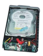
4. Turn the enclosure so that the bottom side is facing up and insert the first screw. Tighten the first screw ensuring that proper alignment is maintained while tightening. Repeat for the three screws.
