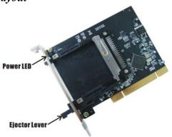
**Note:** The ejector lever can be placed in two positions, locked and unlocked. When inserting a PC Card, the lever can be in either position. However, the lever must be in the unlocked position to eject a PC Card. To unlock the lever, push it until you hear a click then release it.
