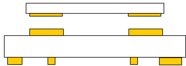
Figure 20. Correct PCB Top Metal Pattern Under Package
