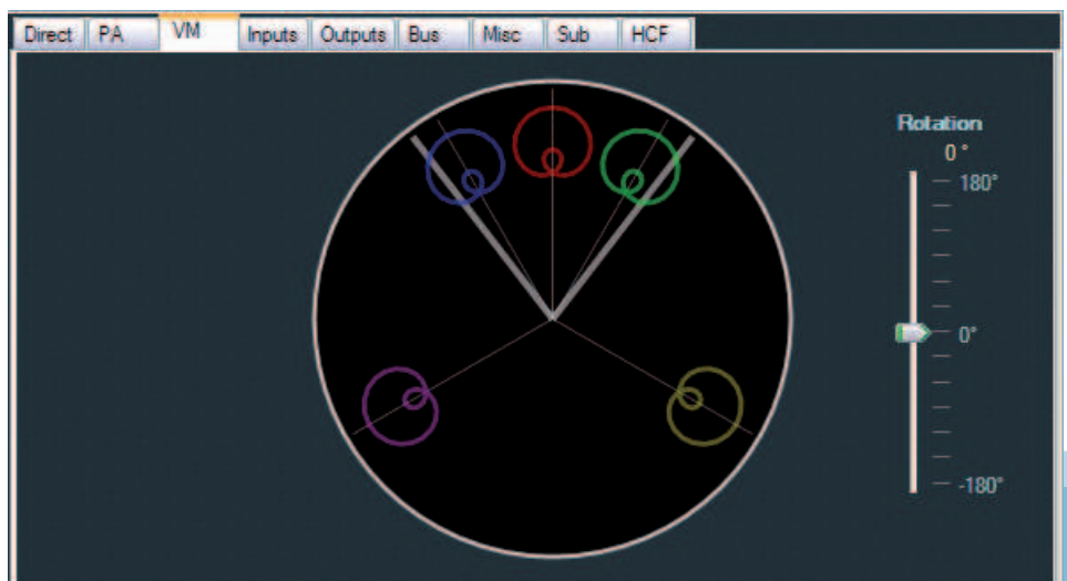
The virtual microphones are shown on a surround circle. You can adjust the acceptance angle, the polar pattern, and the distance between the microphones.
