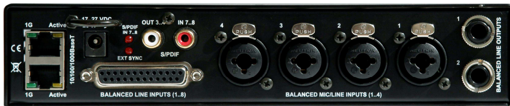
Rear panel with connectors of AUBION X.8
