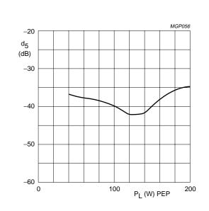
Class-AB operation; V<sub>DS</sub> = 28 V; I<sub>DQ</sub> = 1 A; R<sub>GS</sub> = 9.8  $\Omega$ ; f<sub>1</sub> = 28.000 MHz; f<sub>2</sub> = 28.001 MHz.
