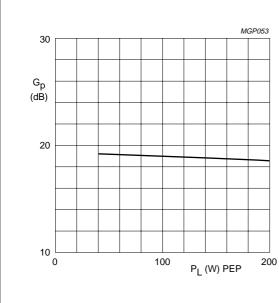
Class-AB operation;  $V_{DS}$  = 28 V;  $I_{DQ}$  = 1 A;  $R_{GS}$  = 9.8  $\Omega$ ;  $f_1$  = 28.000 MHz;  $f_2$  = 28.001 MHz.
