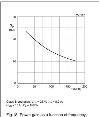
Fig.18 Power gain as a function of frequency typical values.
