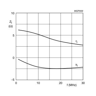
Class-AB operation; V<sub>DS</sub> = 28 V; I<sub>DQ</sub> = 1 A; R<sub>GS</sub> = 6.25  $\Omega$ ; P<sub>L</sub> = 150 W (PEP); R<sub>L</sub> = 2.1  $\Omega$ .
