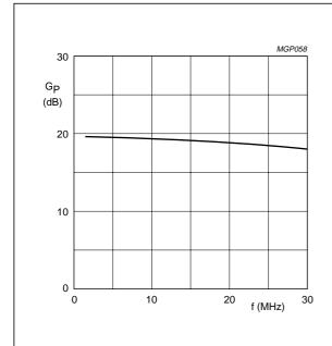
Class-AB operation;  $V_{DS}$  = 28 V;  $I_{DQ}$  = 1 A;  $R_{GS}$  = 6.25  $\Omega$ ;  $P_L$  = 150 W (PEP);  $R_L$  = 2.1  $\Omega$ .
