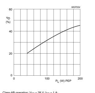
Class-AB operation;  $V_{DS}$  = 28 V;  $I_{DQ}$  = 1 A;  $R_{GS}$  = 9.8  $\Omega$ ;  $f_1$  = 28.000 MHz;  $f_2$  = 28.001 MHz.
