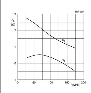
Class-B operation; V<sub>DS</sub> = 28 V; I<sub>DQ</sub> = 0.2 A; R<sub>GS</sub> = 15  $\Omega$ ; P<sub>L</sub> = 150 W.
