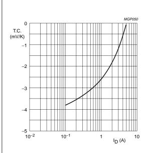
$V_{DS}$  = 28 V; valid for  $T_h$  = 25 to 70  $^{\circ}C.$
