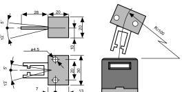
Adjustable, flexible key supplied with 'F3' models. The tongue can be adjusted in four directions for doors of small dimensions where the door radius is down to 100mm.
