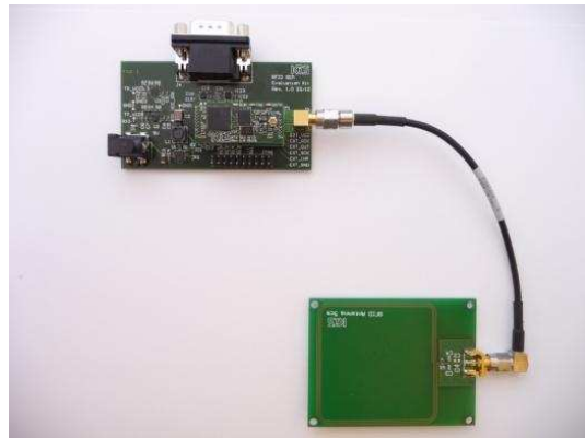
Picture 4 – exemplary arrangement: Evaluation kit with RFID OEM module and 5cm PCB RFID antenna
