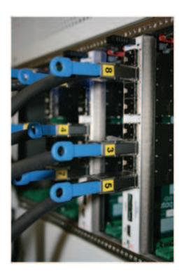
Nutaq RRHs and Octal V6 Baseband Core modules are interconnected using cabled link technology that supports multiple communication topologies and which are user-defined, adaptable and scalable to multiple baseband processing schemes. This provides the TitanMIMO testbed with almost infinite flexibility and reduces risks associated with fixed solutions that can't be adapted and can't scale (see next section model examples).
