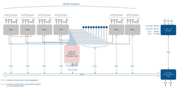
Note: A 128 transceiver testbed built combining 16x RRH and aggregating all channels to a master octal V6 baseband processing core.
