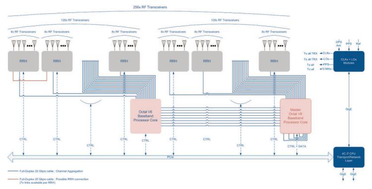
**Note**: A 256 transceiver testbed built combining 32x RRH and aggregating all channels to 2x octal V6 baseband processing core where a master core does the final aggregation.
