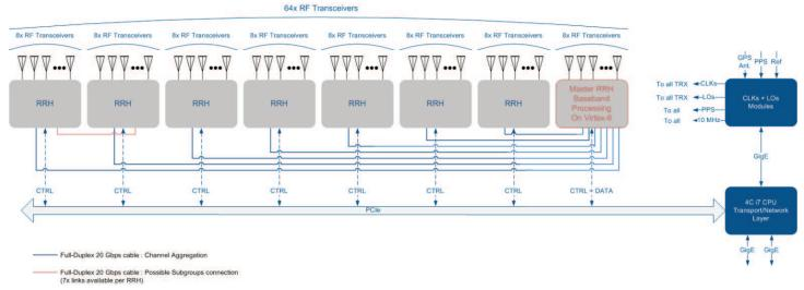
Note: A low cost 64 transceiver testbed built combining 8x RRH and aggregating all channels to a master RRH for baseband processing.
