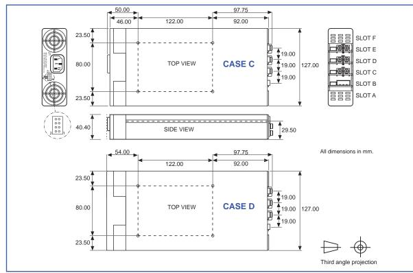
Mounting Holes 4 x M4 threaded holes on Base. Max screw penetration is 6mm from Base.
