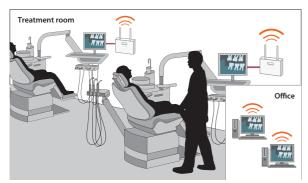
The monitor next to the treatment chain is wirelessly connected to the PC in the office, so that patient files and X-rays can be called up there. This means that there is no need to set up a PC next to each treatment chair, which has a positive effect on the room design.
