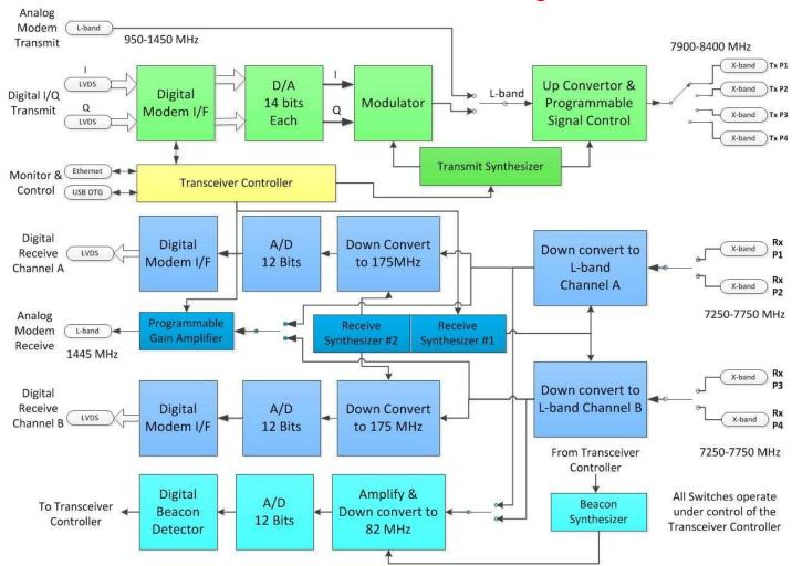
The Alico RF transceiver comprises of a single superheterodyne transmitter, dual super-heterodyne receiver channels and a Beacon receiver. Figure above illustrates the RF Transceiver functional block diagram
