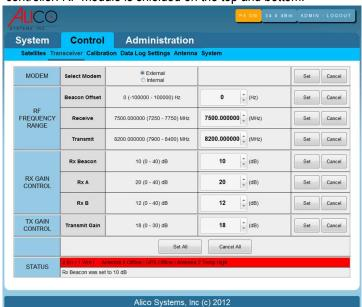
Ethernet based Monitor and control interface provided by a standard browser. Transceiver includes a HTTP web server which supports provisioning and transceiver management including data logging and configuration save and reload capability. On board flash stores configuration when powered off.
