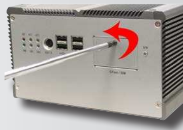
Loosen the screw and open the door
