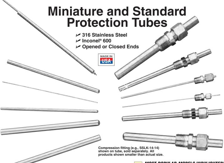
NEWPORT® miniature and standard protection tubes are available in 316 stainless steel and Inconel 600 nickel alloy. Tubes are available either opened at both ends or with one end closed. Standard length available from stock is 150 mm (6"); however, practically any length tube is available on short delivery.
