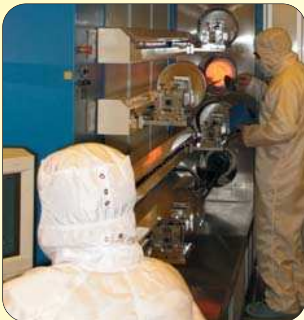
Super OMEGACLAD® XL thermocouple probes in its Class 10 clean rooms to monitor critical process temperatures and achieve consistent, high-quality products.
