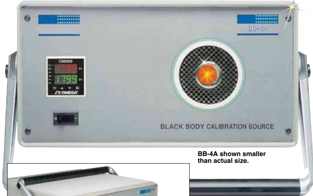
Shown calibrating the OS1552-A pyrometer. Visit newportUS.com for details.
