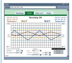
The iSD can display and chart absolute measurements in two locations and a differential measurement between the two locations.
