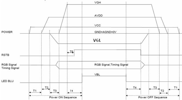
Note: T1≥20ms, T2≥20ms, T3≥5ms, T4≥100ms, T5≥5ms.
