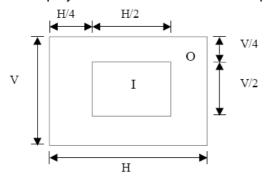
Note5: Polarizer bubble is defined as the bubble appears on active display area. The defect of polarizer bubble shall be ignored if the polarizer bubble appears on the outside of active display area.
