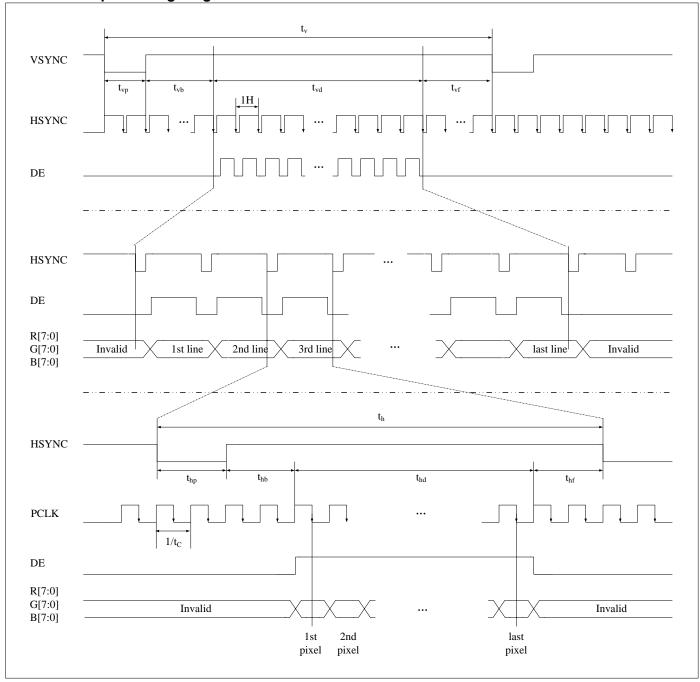
Note 1: When DE is pulled low, Sync mode is active using HSYNC+ VSYNC for timing control. Note 2: When DE is pulled high for active data and pulled low for blanking data, DE mode is active for timing control.
