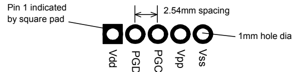
Figure 13. Recommended plate-through connector design
