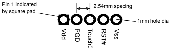
Figure 4. Recommended plate-through connector design
