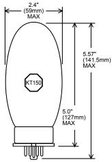
GLASS BULB LARGE WAFER OCTAL WITH BARRIERS 7 PIN LOW LOSS B7-99 FOR AUDIO SERICE APPLICATIONS
