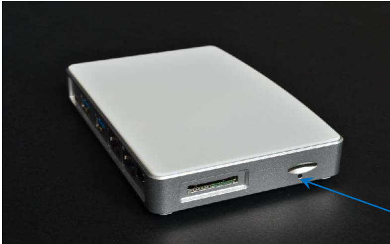
6、GPIO reset button hole.
