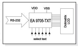
All displays feature LED-backlight illumination. Matching frontal bezels with antiglare glass is included also. With accessories cable EA KV24-9B (aro. 1,50m) the EA 9705-TXT can be plugged directly into the 9-pin. SUB-D socket of a PC.
