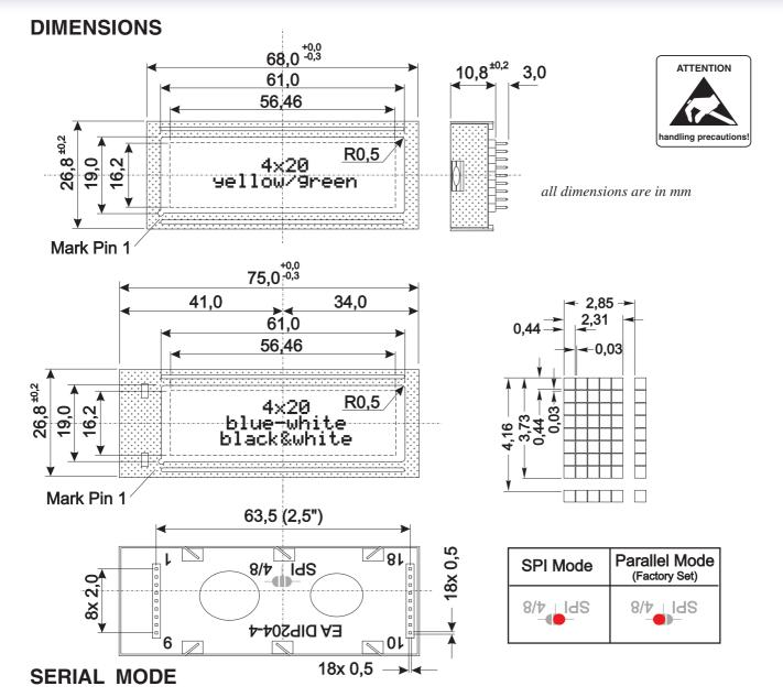
Factory set for interface is parallel with 4 bit or 8 bit data bus. Alternative module can be programmes with serial data stream. For that solder link **4/8** has to be opened and closed to **SPI** side. Specification for serial operation mode is written down in user manual for KS0073: <a href="http://www.lcd-module.de/eng/pdf/zubehoer/ks0073.pdf">http://www.lcd-module.de/eng/pdf/zubehoer/ks0073.pdf</a>
