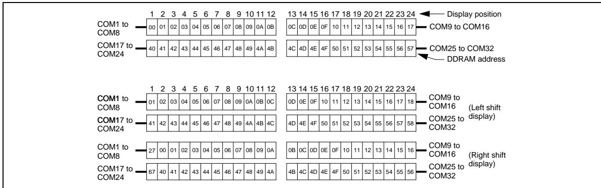
Figure 5 2-Line by 24-Character Display (5-Dot Font Width)
