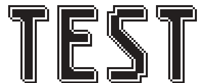
When "outline font" is overlayed again (EXOR) at pos.2,2. than the result is an "outline font with black filling".
