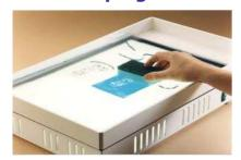
Once exposure is complete take out the artwork and lay on the illuminated light box. Then place the sloped processing tray on top of the light box.
