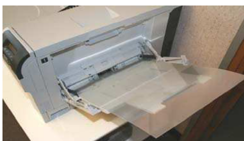
Load in bypass Tray
