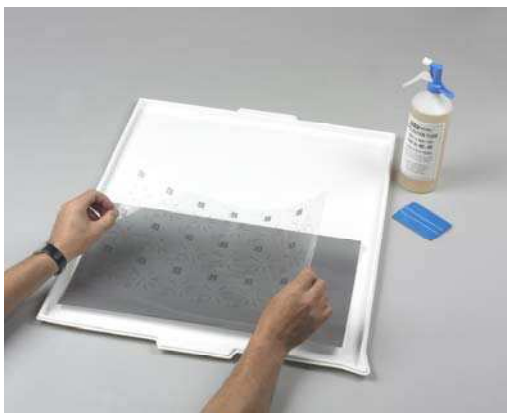
Laying the Laser Film
