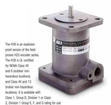
in hazardous locations. It features a standard shaft seal, double bearing seals, and a cast aluminum housing with hard anodized and dichromate sealed finish. The H38 is suitable for use in petroleum service industries, solvent refining operations, spray painting applications, and explosive dust environments.
