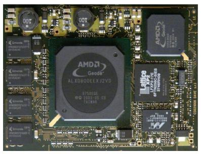
**NEPTUNE** is a ready-to-use CPU module based on AMD Geode LX x86 compatible microprocessor family.
