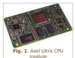
Axel is the new top-class Solo/Dual/Quad core ARM Cortex-A9 CPU module by **DAVE Embedded Systems**, based on the recent Freescale i.MX6 application processor.
