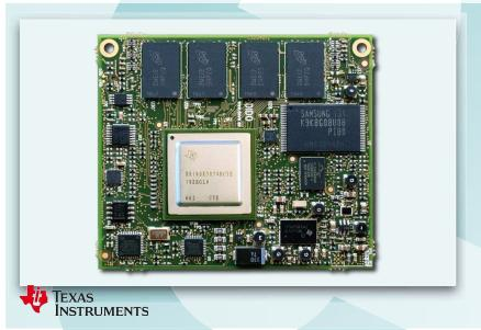
DIDO has an extended connectivity thanks to PCIe, dual CAN, Ethernet, SATA and native 3.3V I/O, sophisticated displays with HD Video Encoding/Decoding Capabilities (HDVCIP) and rich user-interfaces.
