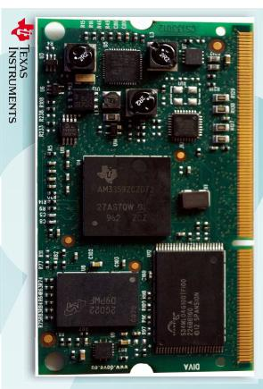
DIVA is a ready-to-use CPU module by DAVE Embedded Systems, based on Texas Instruments Cortex-A8 application processor from AM335x (Sitara) family.
