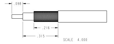
TRIMMING DIMENSIONS FOR RG-58 CABLE
