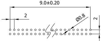
Recommended P.C. Board Tolerances: ±0.05mm Hole Layout
