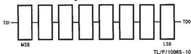
Instruction Register Scan Chain Definition
